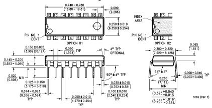
Molded Dual-In-Line Package (N) Order Number MM74HC221AJN NS Package Number N16E
