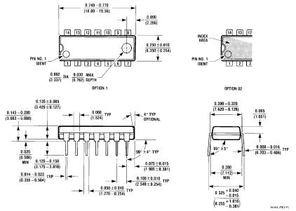
14-Lead Molded Dual-In-Line Package (N) Order Number DM7411N NS Package Number N14A
