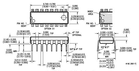
16-Lead Molded Dual-In-Line Package (N) Order Number DM74LS195AN NS Package Number N16E
